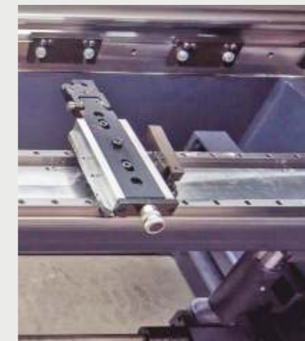
Double Linear Guided Stronger Back Gauges
