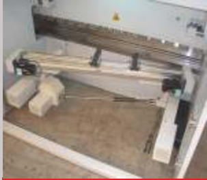
X1-X2-R-Z1-Z2 Type Back Gauge
